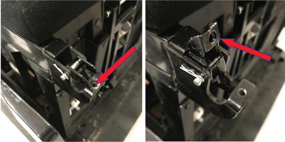
Make sure to install the axle bushings onto the axles on the legrest before placing the legrest on the chair:
