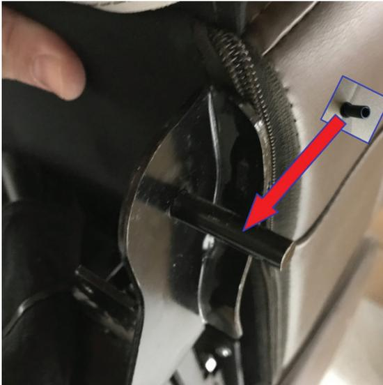
Now place the legrest axles on the axle holders, lower the latch, and install the Phillips screws.
