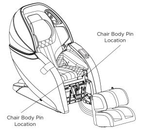
Slide Hinge over Pin on each side Pin Hinge
