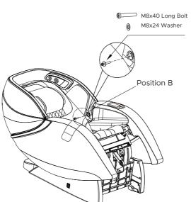
Step 8: Locate the shorter, black M8 Bolts (2) and Washers (2) from the Accessory Box. Fasten
