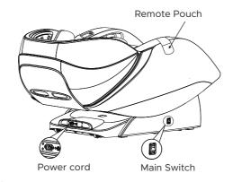
Plug the chair into a grounded electrical outlet. Power on the Main power switch and press the Power button on the remote until the chair uprights out of shipping position. (you may need to press power more than once).
