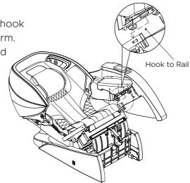
Pin retainer Next locate the Pin in position A on the Arm and secure it under the Pin Retainer on the Chair body in position A from step 3. Slide Pin under Retainer to secure
