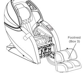
Air nozzle ◀ ▶ Air hose Footrest drive Footrest drive connector plug connector port Footrest power 4 Footrest power connector port connector plug Footrest air Footrest air valve connector port connector plug
