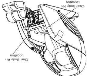
Remove Clips from Body Pins by sliding up
